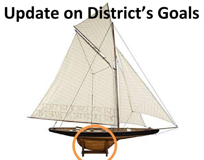
The keel is basically a flat blade sticking down into the water from a sailboat's bottom. It has two functions: it prevents the boat from being blown sideways by the wind, and it holds the ballast that keeps the boat right-side up.
