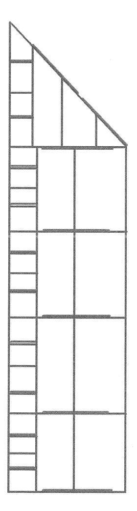
Ceiling diagram for placement of baffles. 10 baffles - 3' x 8' 7 baffles - 4' x 8'
